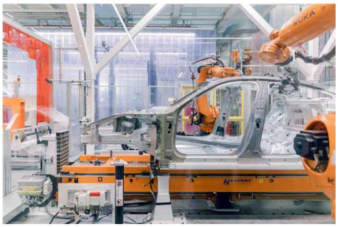
The construction line for the Audi e-tron GT body uses correlation-free measuring techniques that, for example, perfect the dimensional accuracy of gap measurements.
